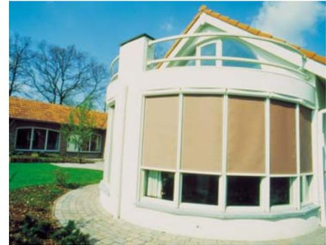
The SC2000 Mastershade® is an exterior vertical rolling screen system which can be rolled up and down as needed. The fabric runs inside vertical guide Tracks or Cable Guides by means of gravity. When the shade is retracted the fabric is stored in the built-in protective box. A specially designed horizontal weighted Hem bar keeps the fabric taut. The Mastershade® is made of the highest quality extruded aluminum. The SC2000 has a 4" Cassette box.
