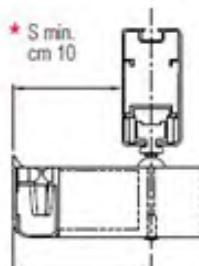
\*With Tie rods max projection is 5m or 16' 5" projection. Must be bolted to structural wall
