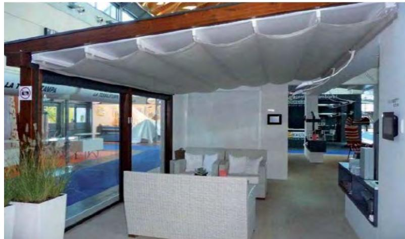
To create a nice atmospheres with wall Pergola® Awnings , it is possible to apply an "Undercover" installed under the ribs. Please note fabric will hang lower than top Vinyl cover. This undercover will be slightly narrower than the top cover by at least 4" / 10 cm per side to prevent water from going up along the PVC flap and wet the fabric of the under cover (Solid 60" fabric colors only).
