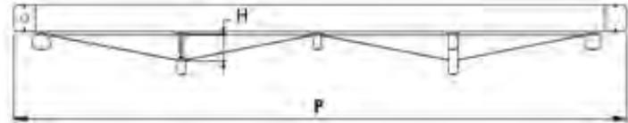
OPTION D: “V” Cut alternating panels for Type 1 Pergola® only. Max width is 5 meters x 9 m projection
