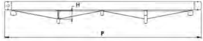
OPTION D: “V” Cut alternating panels for Type 1 Pergola® only. Max width is 5 meters x 9 m projection
