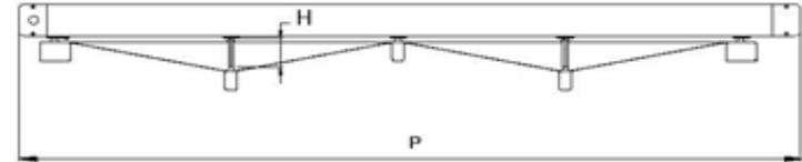
OPTION D: “V” Cut to one side only. For Type 1 Pergola® only. Max width 5 meter x 9 m projection.
