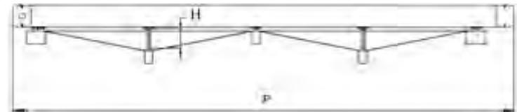
OPTION F: “V” Cut to both sides. For Type 2 Pergolas only. Max width 7 meters x 9 m projection
