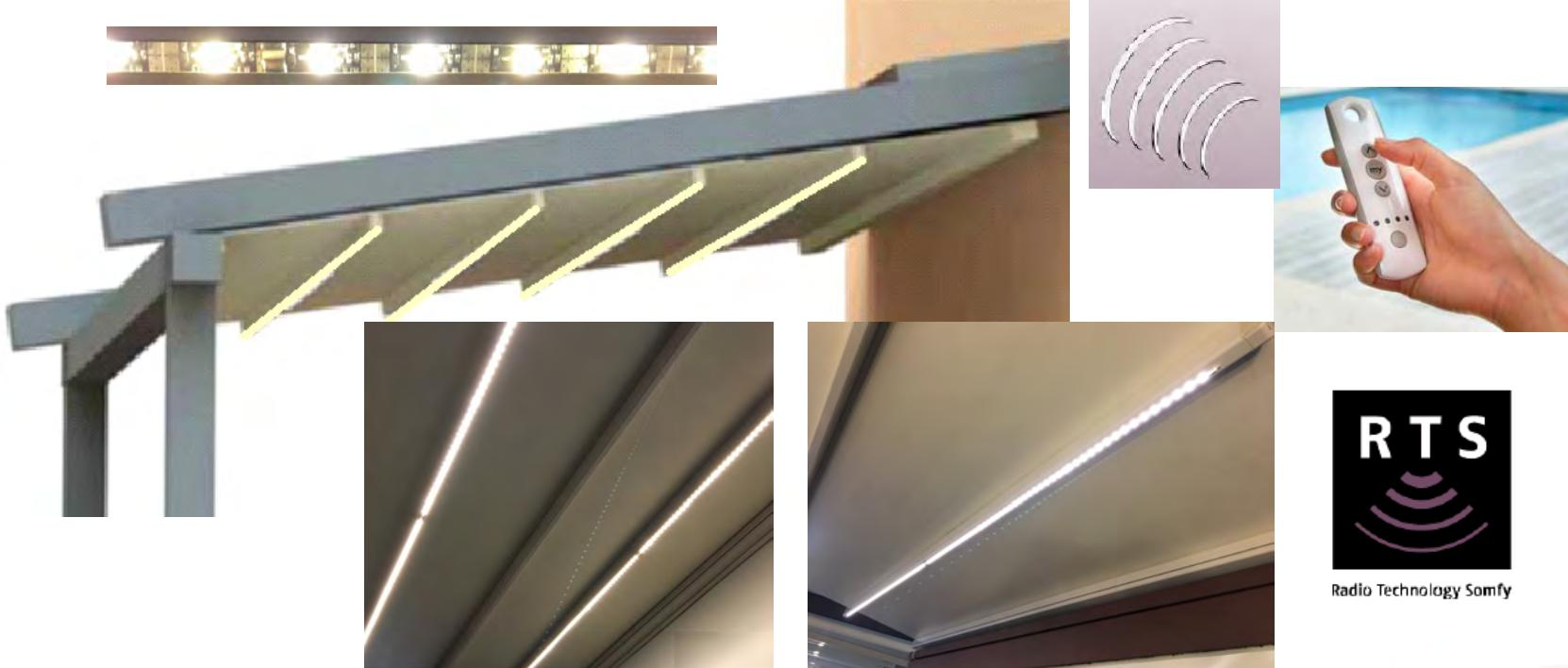
The soft white LED lighting strips are available up to 40 ft long (Maximum allowable amount of linear lighting per Somfy Lighting receiver). One Somfy lighting receiver #1811486 is needed per 40 ft. of linear LED lighting. Typically two to four ( 2 - 4) lighting bars are centered per each bay or section of Pergola. Multi Channel Telis remotes are needed for the LED lighting depending on how many lighting receivers are needed.
