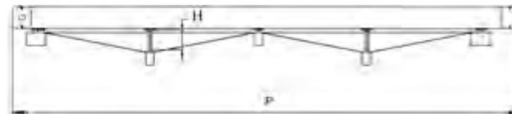
OPTION F: “V” Cut to both sides. For Type 2 Pergolas only. Max width 7 meters x 9 m projection
