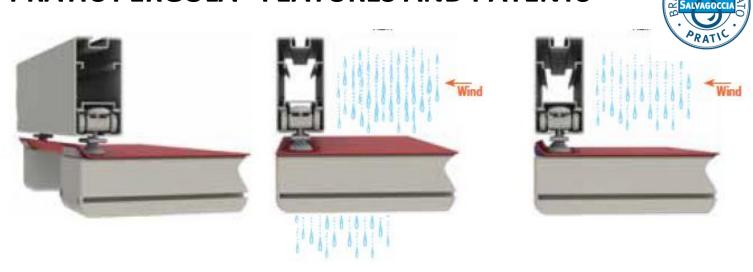
The patented "drop catcher" system keeps water from flowing off the sides when the wind is pushing water sideways. Instead the water will flow off the front or into the gutter.
