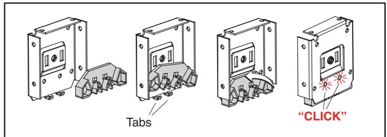
When using the SL-10 with fascia brackets and panel, install the shade and route the control cord/bead chain through the front two channels as usual. Snap the diverter cover on the chain diverter as shown.
