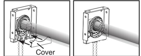
**4 Inch Fascia:** Chain diverter is not required on 4 inch Fascia.
