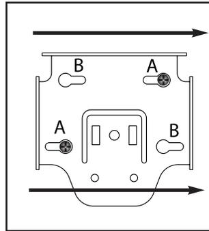
3.) Slip the mounting bracket over the two screws and slide the bracket sideways until the screws heads capture the bracket.
