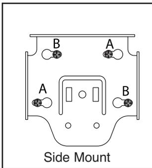
5.) Install additional screws in the additional two holes if required.
