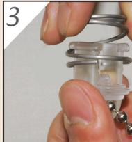
3 Squeeze guide legs while sliding spring over guide completely. (Be sure spring is all the way over the legs of the guide).
