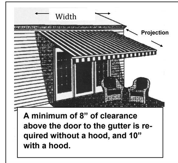
The SUNAIR® Lateral Arm Awning is designed for residential decks, patios and commercial storefronts. Smaller projections should be used for a storefront awning. The awnings are designed for sun protection; they are not designed to withstand wind or heavy rain and should not be sold for such purposes (see warranty).
