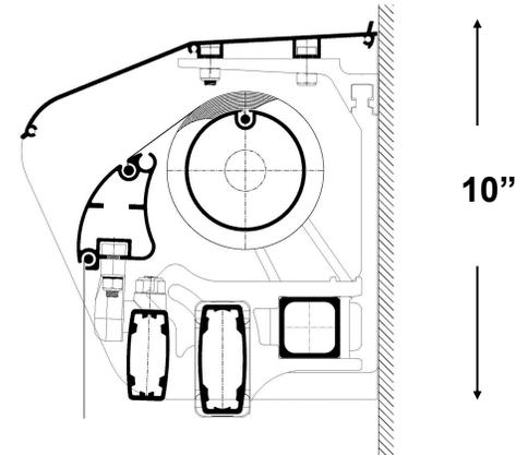
Sunair® offers an optional aluminum one piece hood, made from the highest quality aluminum. The hood protects the fabric when the awning is in retracted position. With the aluminum hood, your awning is always automatically covered when you retract it. If the awning is mounted under an overhang protruding at least 10", then the optional hood is not needed.
