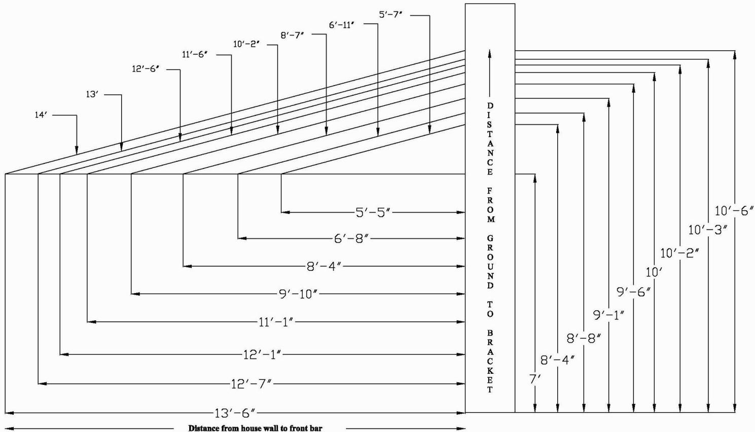
**For example:** The brackets on an awning with 10' projection needs to be mounted 9'6" from the ground on a residential installation,  $10' \times 3" = 2'6"$  &  $2'6" + 7" = 9'6"$ ). Because the ideal pitch may not always be attained, it is possible to install the awning lower than the ideal pitch. While the "3/12" rule is ideal, it is perfectly fine to install the awning with a 2/12 pitch. A 1/12 pitch is absolute minimum. Maximum pitch is 45°.
