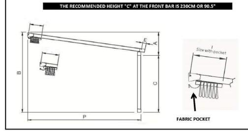
Above are slope requirements are for a LEVEL Pergola® unit with "TAUT" fabric and water drainage to the front gutter. Flat units are possible with added water drainage to sides (optional extra charge). Required slope varies with Pergola model. Free standing Pergola® units that are flat and do not need a slope.
