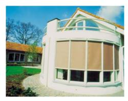
The SC2000 Mastershade® is an exterior vertical rolling screen system which can be rolled up and down as needed. The fabric runs inside vertical guide Tracks or Cable Guides by means of gravity. When the shade is retracted the fabric is stored in the built-in protective box. A specially designed horizontal weighted Hem bar keeps the fabric taut. The Mastershade® is made of the highest quality extruded aluminum. The SC2000 has a 4"Cassette box.
