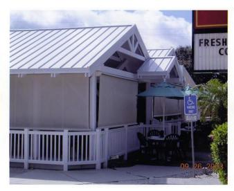
The SC1000 & SC1500 Mastershade® are two simple economical exterior cabled vertical rolling sun screen systems, which can be rolled up and down as needed. The fabric hem bar runs on cable guides by means of gravity. When the shade is retracted the fabric is stored in the built-in protective box on SC1500 unit (SC1000 unit is an open roller). A galvanized steel painted weighted bar in the fabric fold / pocket keeps the fabric taut.
