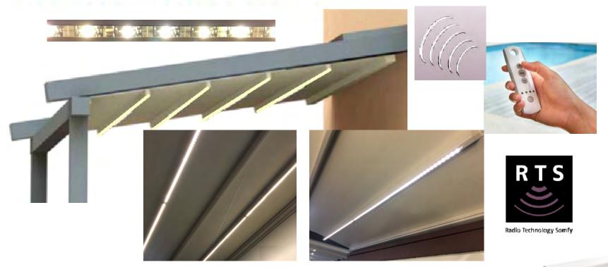
The soft white LED lighting strips are available up to 40 ft long (Maximum allowable amount of linear lighting per Somfy Lighting receiver). One Somfy lighting receiver #1811486 is needed per 40 ft. of linear LED lighting. Typically two to four (2 - 4) lighting bars are centered per each bay or section of Pergola. Multi Channel Telis remotes are needed for the LED lighting depending on how many lighting receivers are needed.
