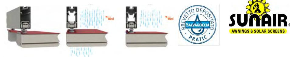
The patented drip catcher keeps water from flowing off the sides when the wind is pushing water sideways. Instead the water will flow off the front or into the gutter.
