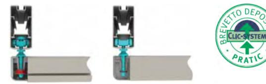
The patented click system allows for easy and safe installation of the fabric and fabric ribs to the frame carriages using an easy click and lock system.
