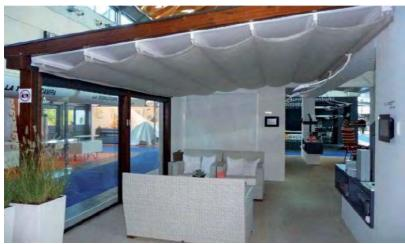
To create a nice atmospheres with wall Pergola® Awnings, it is possible to apply an "Undercover" installed under the ribs. Please note fabric will hang lower than top Vinyl cover. This undercover will be slightly narrower than the top cover by at least 4" / 10 cm per side to prevent water from going up along the PVC flap and wet the fabric of the under cover (Solid 60" fabric colors only).
