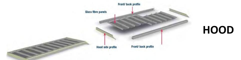
HOOD: Is available standard with fiberglass panels with a metal frame. The metal frame color typically matches the awning frame. Brown fiberglass panels are standard. White fiberglass panels are also available standard but subject to stock availability.
