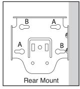
6.) The bracket contains other slotted mounting holes for rear or top mounted shades.
