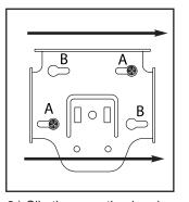
3.) Slip the mounting bracket over the two screws and slide the bracket sideways until the screws heads capture the bracket.
