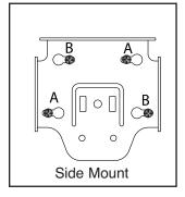
5.) Install additional screws in the additional two holes if required.
