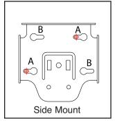
1.) Hold the mounting bracket in position in the window and mark the location where the screws should be positioned in either both A & A locations or B & B locations.
