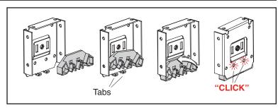
When using the SL-10 with fascia brackets and panel, install the shade and route the control cord/bead chain through the front two channels as usual. Snap the diverter cover on the chain diverter as shown.
