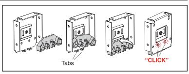
Install the shade and route the control cord/bead chain through the front two channels of the chain diverter. When using SL-10 clutch, snap on diverter cover.
